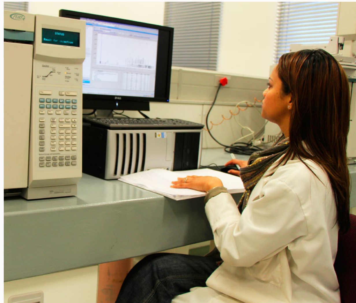
Ms Lynzey Isaacs, Technical Officer in the Chemical Analytical Laboratory, busy with chromatographic analysis of the most important volatile components of wine.
