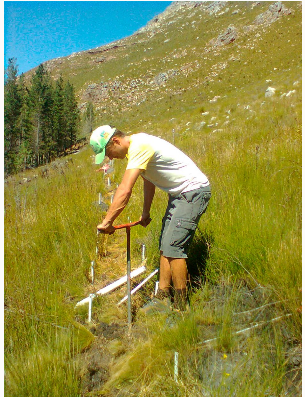
A postgraduate student installing access tubes for a soil water-measuring instrument at Nuweberg.
