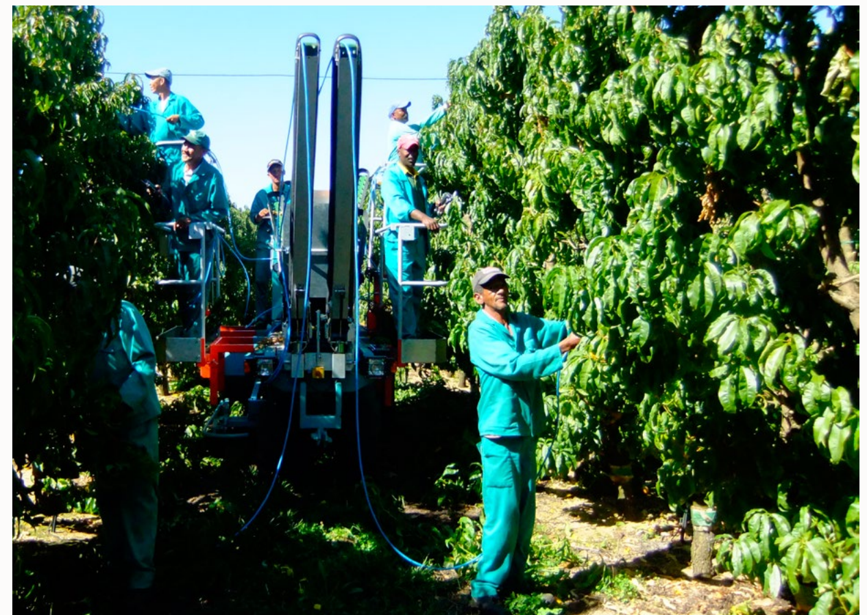
Evaluation of the Hermes harvest system as platform, with air pressure shears for the summer pruning of nectarines.
