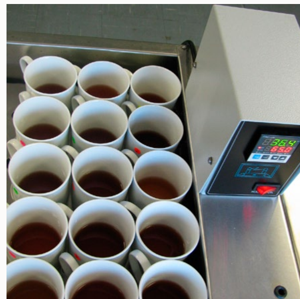
Rooibos tea samples kept in a waterbath to maintain the correct temperature for sensory analyses.
